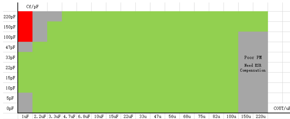
Figure 27. SCT71005 Feed Forward Capacitors recommend( R_2=10k\Omega, V_{OUT}=1.8V )
